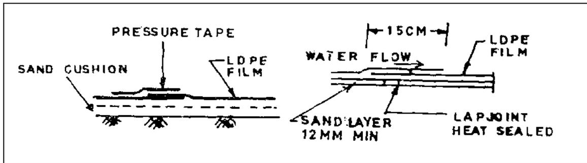
FIG. 11 (v) OVERLAP JOINT WITH PRESSURE TAPE
