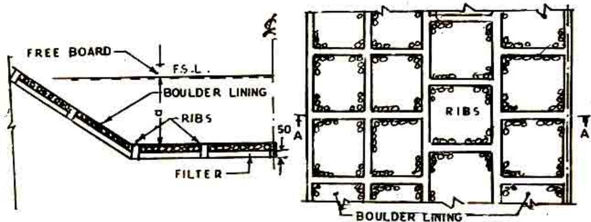
**Fig. 18 Illustratory Layout Of Pitched Lining For Canal**
