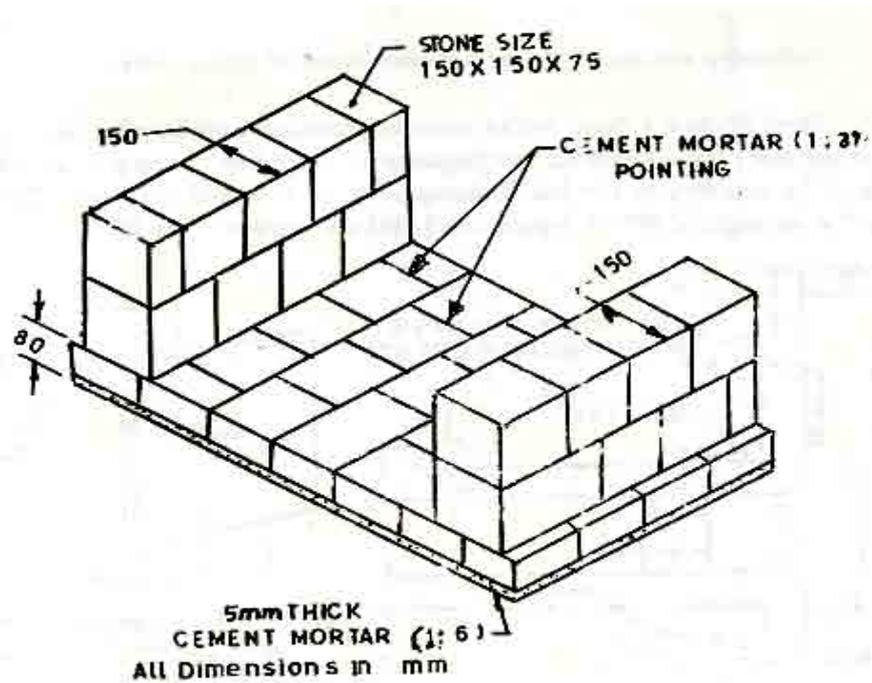
Fig. 23 Stone Masonry Lining
