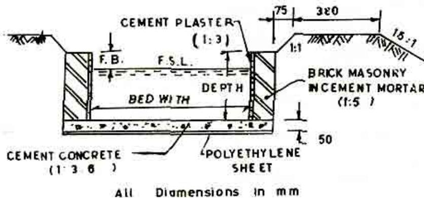
Fig. 21 Typical Cement Concrete And Brick Masonry Section
