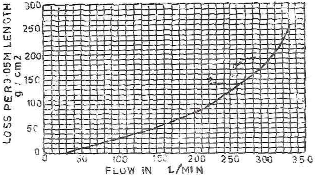
8A : HEAD LOSS PER 3.05 M. LENGTH IN 32 MM PIPE
