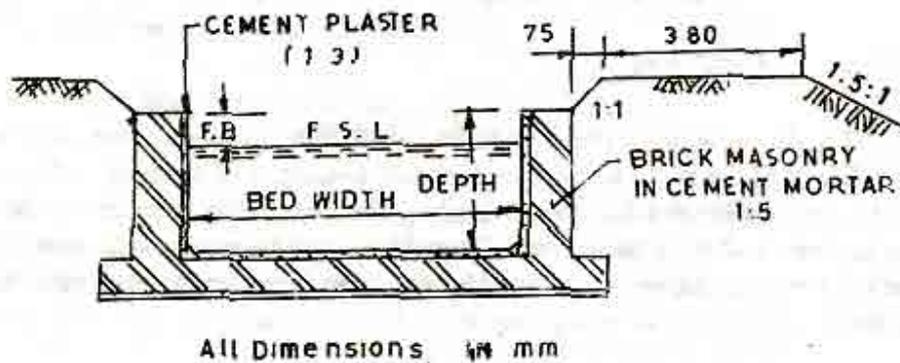
**Fig. 19 Typical Brick Masonry Section**
