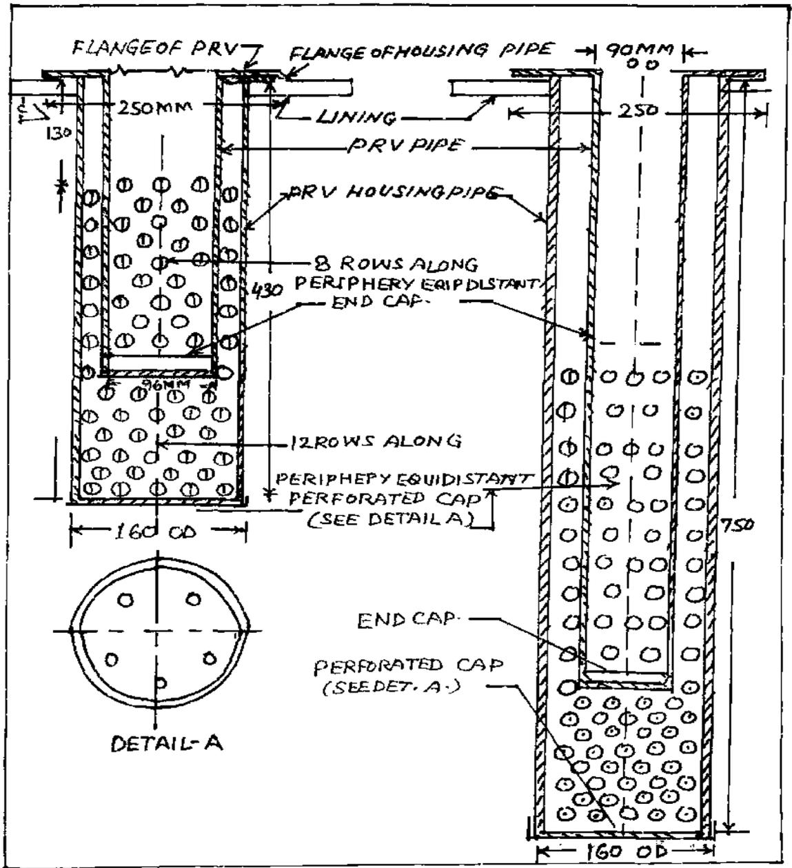
Fig. 7 DETAIL OF PERFORATION IN DRY HOUSING PIPE
