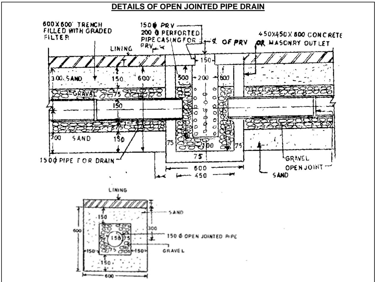
**Fig. 10 DETAILS OF OPEN JOINTED PIPE DRAIN**
