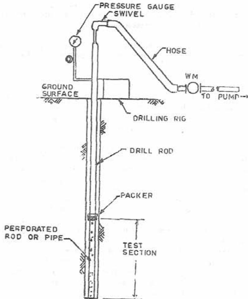
**FIG 7 : SKETCH SHOWING LAYOUT OF EQUIPMENT FOR PERMEABILITY TEST IN DRILL HOLE (SINGLE PACKER METHOD)**
